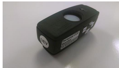
Above: Personal CO 2 sensor worn by astronauts on the International Space Station. (Photo by NASA )
